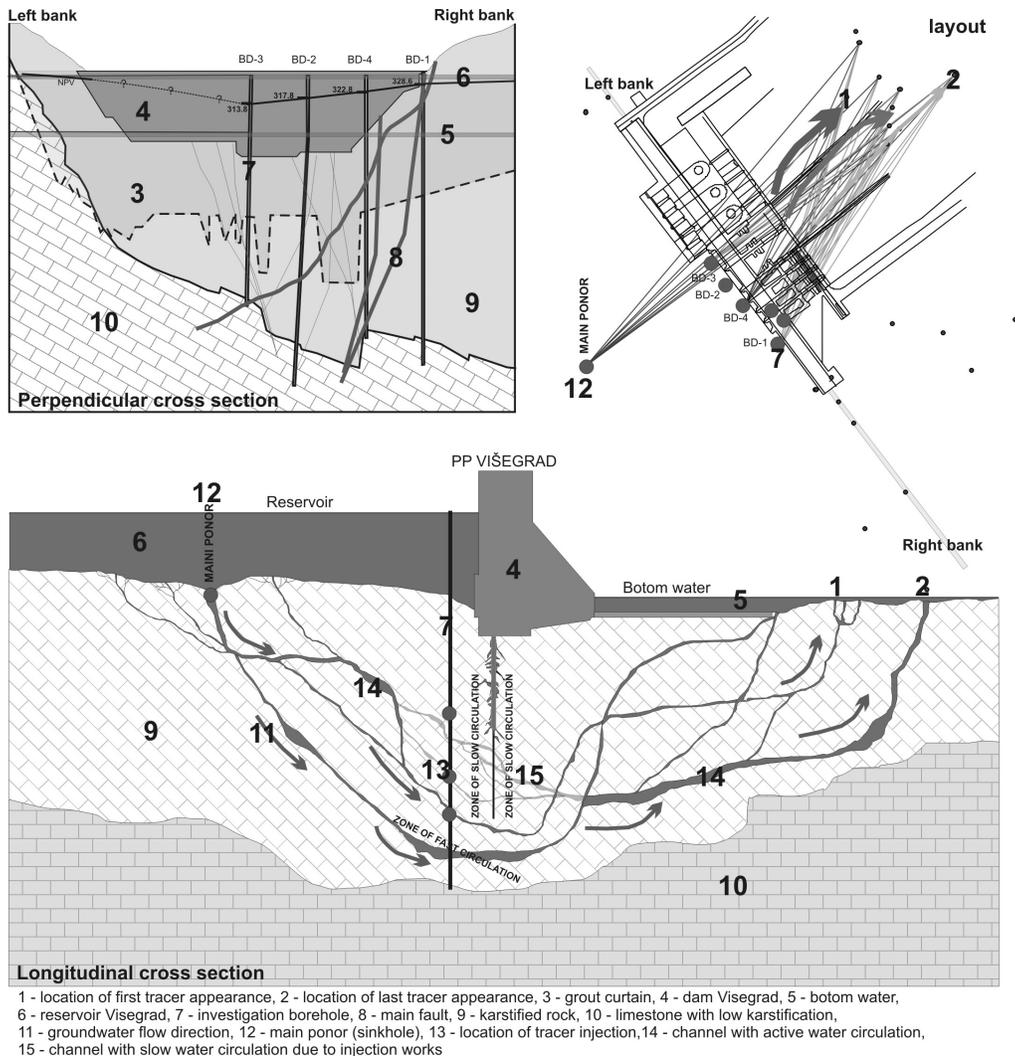
Fig. 2. Hydrogeological characteristic of potential leaking below HPP Visegrad according special investigations conducted in 2009
