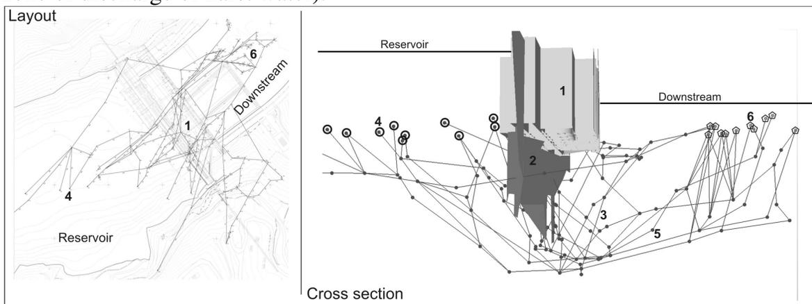
Fig. 3. Spatially-oriented 3D network of potential karst conduits: 1. Dam, 2. Grout curtain, 3. Network - karst conduits - link, 4. Node – sinking zone, 5. Network node – link bifurcation, 6. Discharge zone - springs
