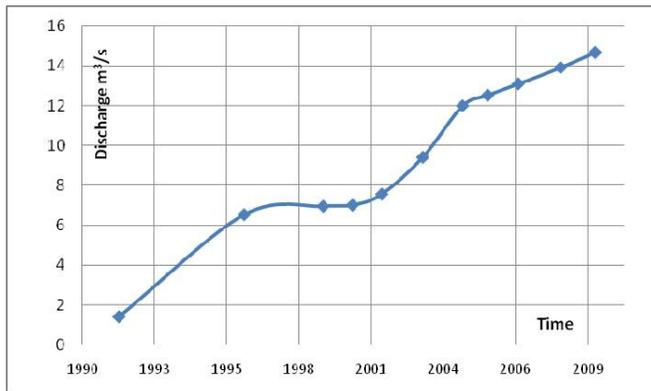
Water seepage beneath the dam was systematically monitored from the year 1991 to the year 2009. Measured values are shown in the graph on Fig. 1.
