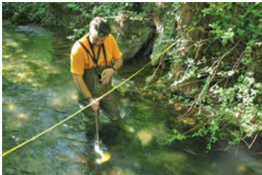
Springflow measurements in Beljanica test area(left) and downloading diver data in Krupac spring (Piro)
