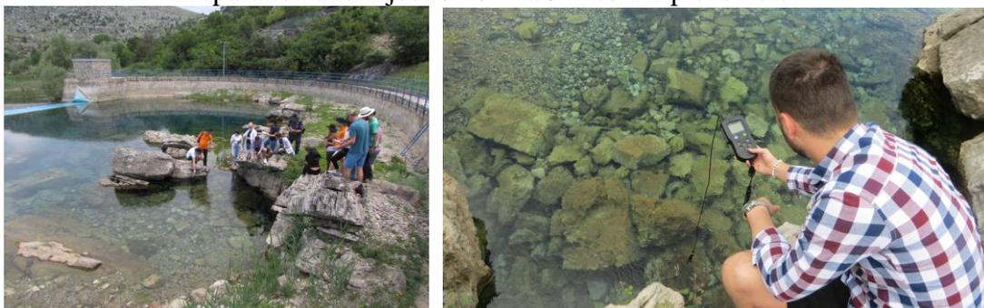
Monitoring of electrical conductivity on the spring
