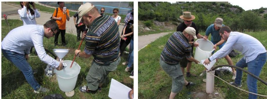
Preparation and injection of NaCl into the piezometer
