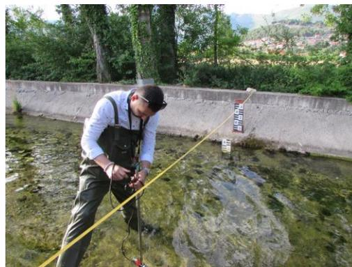
Measurement of spring discharge using current meter
